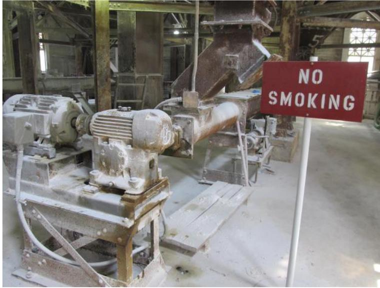
**Figure 3-35: Lime Screw Conveyor**
